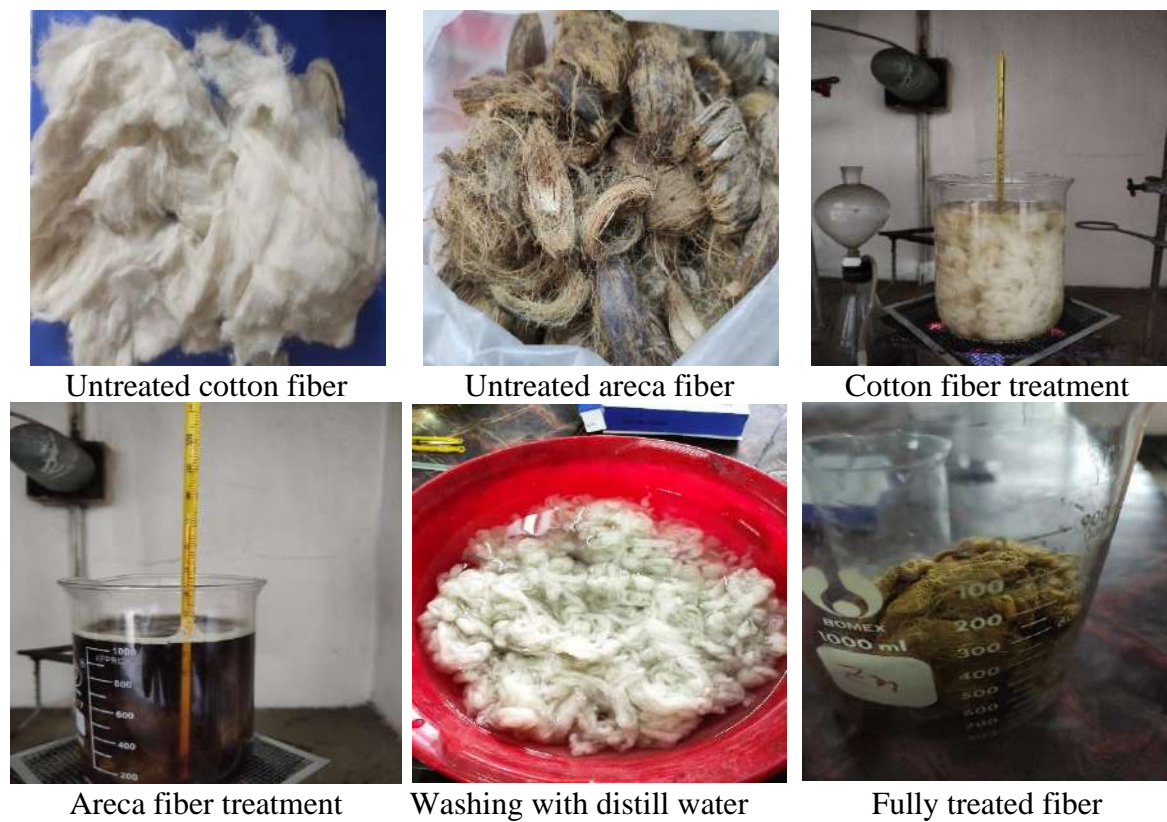
Fig. 3.1 Photographic view of alkali treatment of cotton and areca fiber
