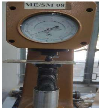
Fig: 4.4 Hardness testing with Rockwell hardness tester (R scale)
