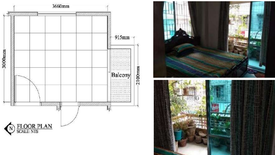
Figure 3. 14: D 1200 bedroom plan; bedroom and balcony interior photos
