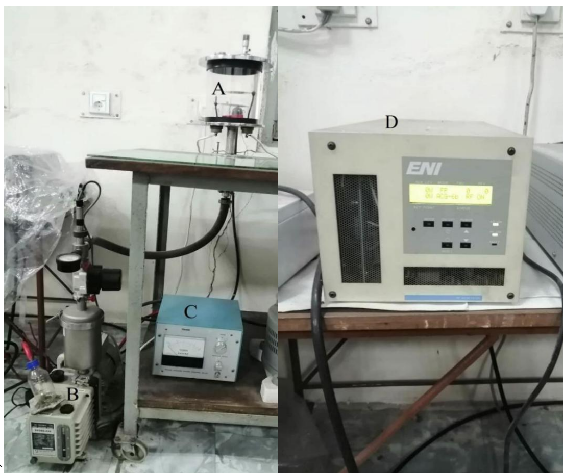
Fig. 3.6 The experimental setup of an RF plasma system (A) Glass chamber, (B) Rotary pump, (C) Pirani gauge and (D) RF generator.
