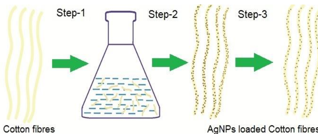
Fig. 3.8 Schematic diagram of fabrication of AgNPs incorporated cotton fibres.
