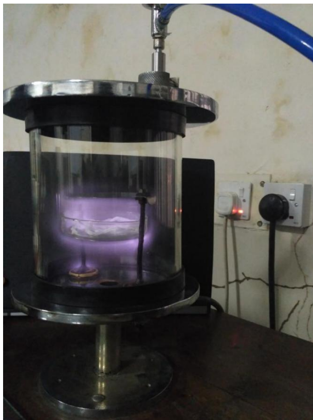
Fig. 3.7 Oxygen plasma treatment process of cotton fibres.
