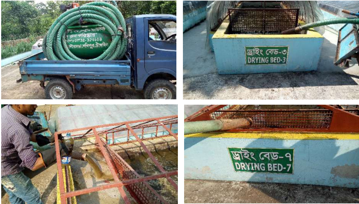
Figure 3.2: Raw sample collection at Sakhipur FSTP prior to discharge into the unplanted drying bed.
