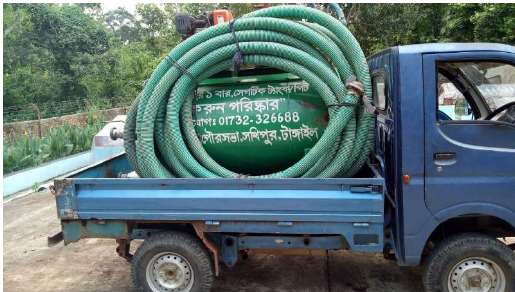
Figure 2.3: Vacutug is used in Sakhipur for collection and transportation of FS
