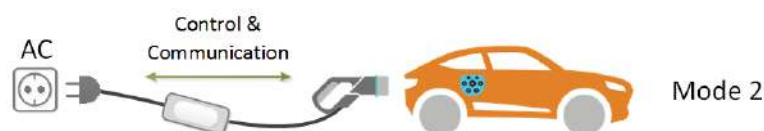
Figure 2.2: Mode 2 EV charging process [13].
