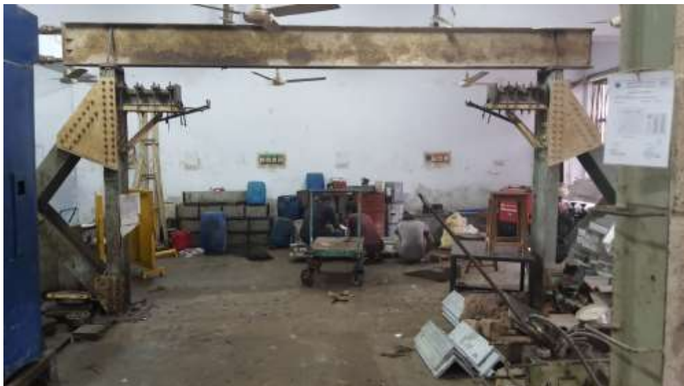
Figure 3.15 Full frame for testing with mounted strong beam at top
