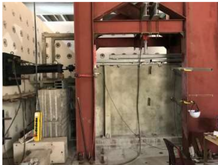
Figure 2.33 Masonry wall sample ready for testing (Hasnat et al., 2022)
