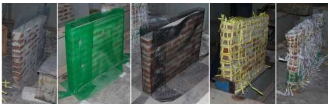
Figure 2.34 Wrapping walls with different mesh, (a) Steel mesh, (b) Soft polymer, (c) Geo-grid, (d) PP-band, (e) Plastic bag (Nissanka et al., 2015)
