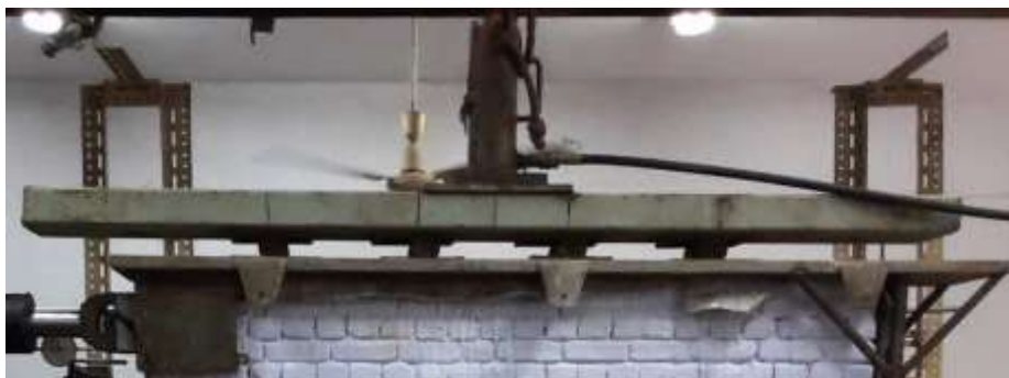
Figure 3.17 Arrangement for vertical and lateral load for wall samples
