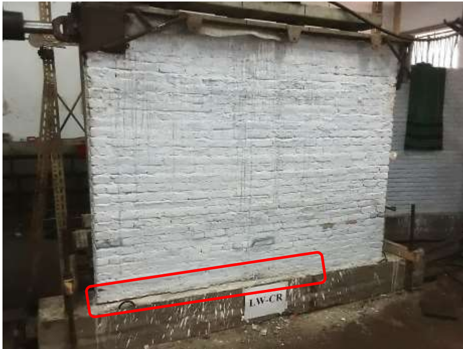
Figure 4.8 Rocking type of failure in LW-CR sample
