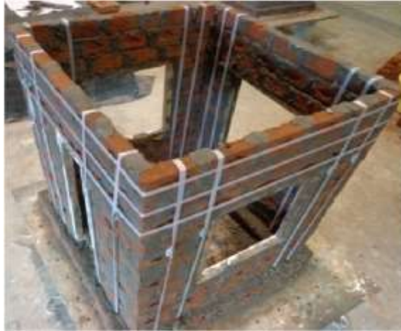
Figure 2.35 Application of PP bands on room (Nayak and Dutta, 2016)
