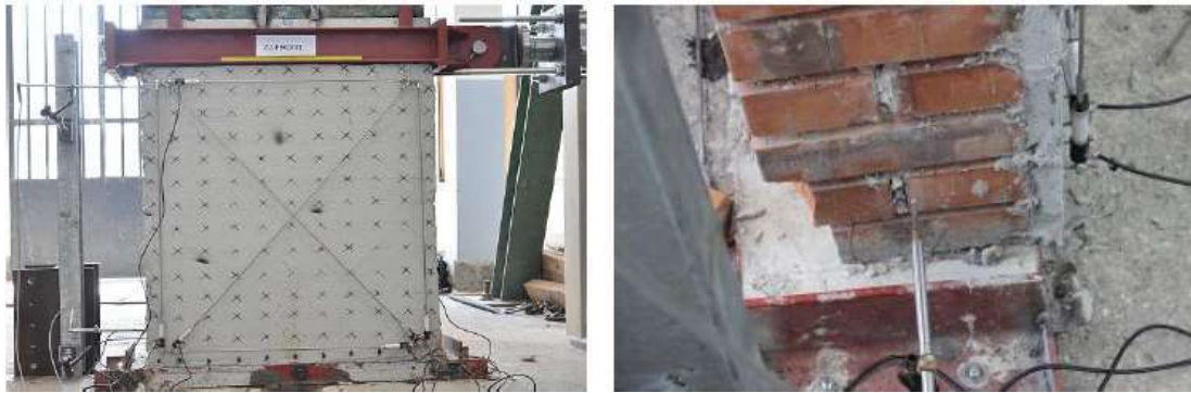
Figure 2.42 Failure mode of strengthened samples (Mustafa et al., 2018)
