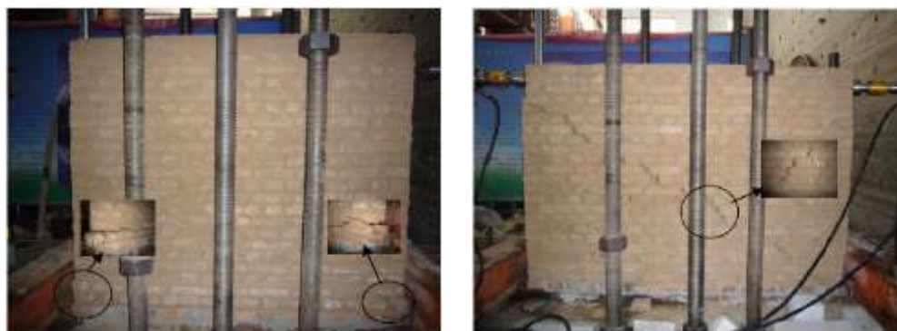
Figure 4.43 Failure mode of URM walls (Feng et al., 2017)
