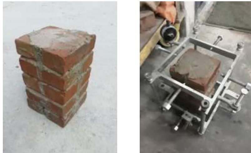
Figure 3.14 Masonry prism samples ready for testing
