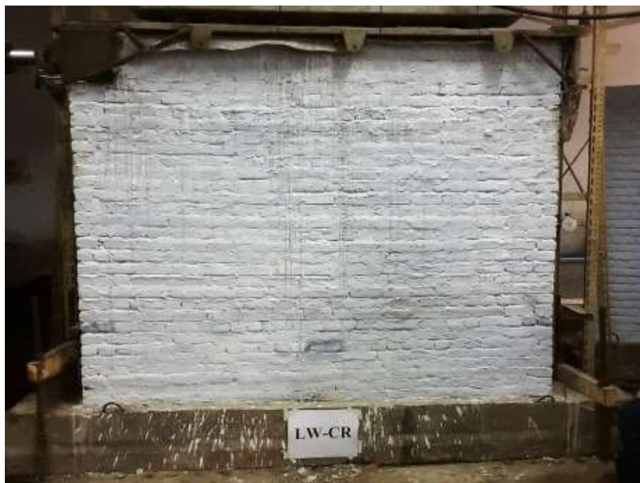
Figure 4.7 LW-CR wall sample before testing
