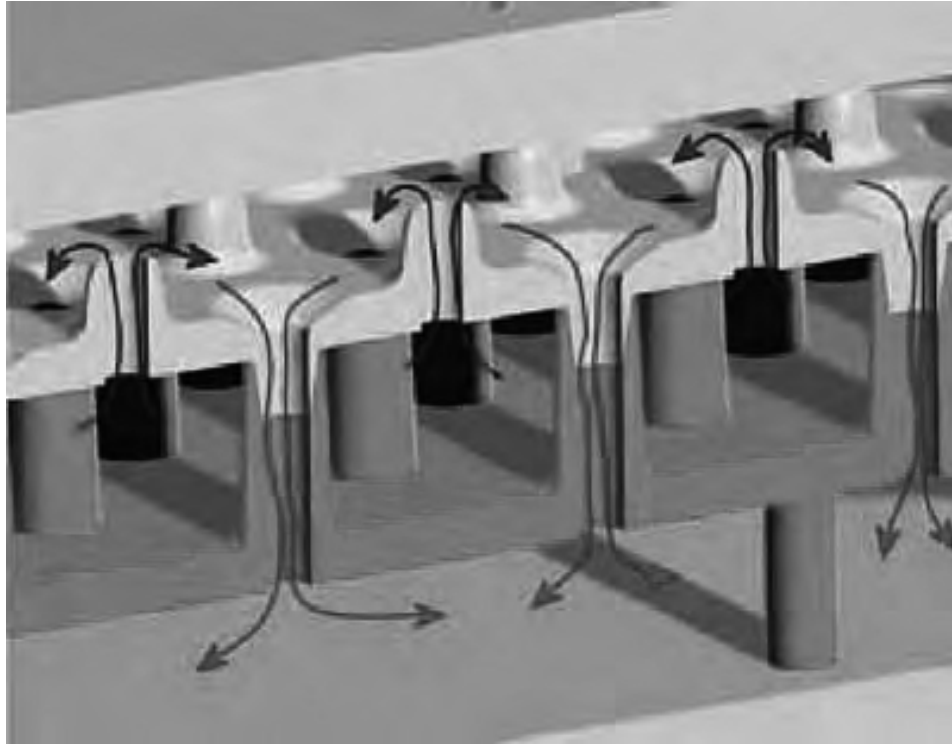
Figure 1.2 Commercially available multiple jet impingement liquid cooling [3]
