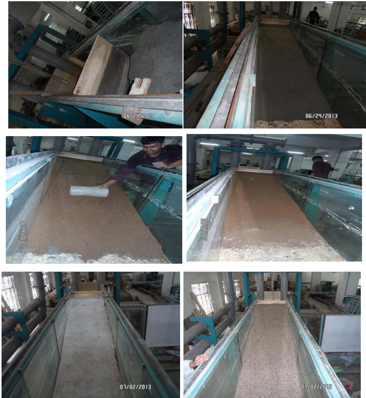
Fig 3.4 Some photographs of slope preparation
