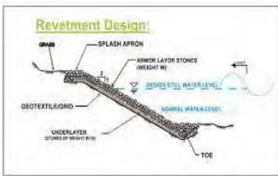
Fig 2.8 Design of revetment
