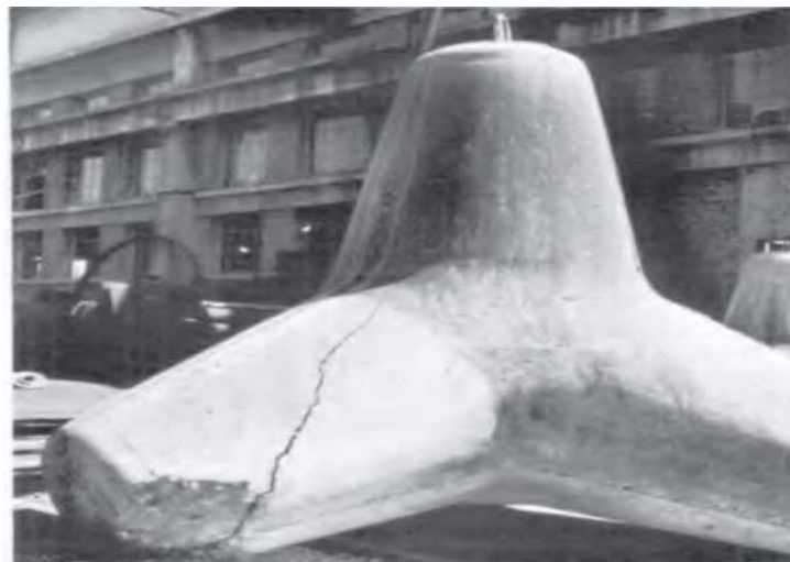
Fig 2.15: A four tone tetrapod after 3 ft. fall
