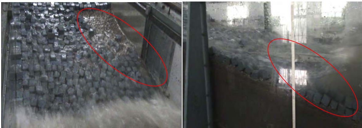
Fig. 4.56 Revetment was unstable after Run No 8 (case-2, T=2.0 sec)
