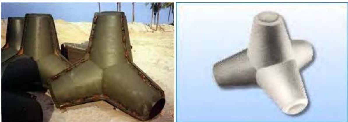
Fig 2.13: Dice for manufacturing Tetrapod
