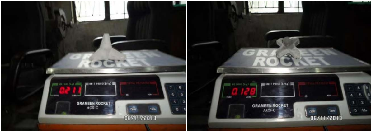
Fig 3.11: Weight of tetrapod and x-block is found same as its design weight
