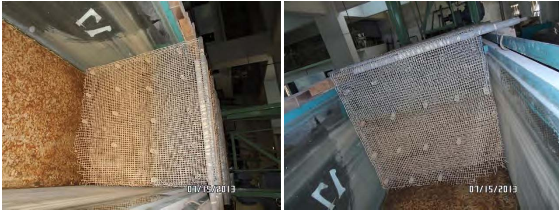
Fig 3.3: Screen for wave re-reflection control
