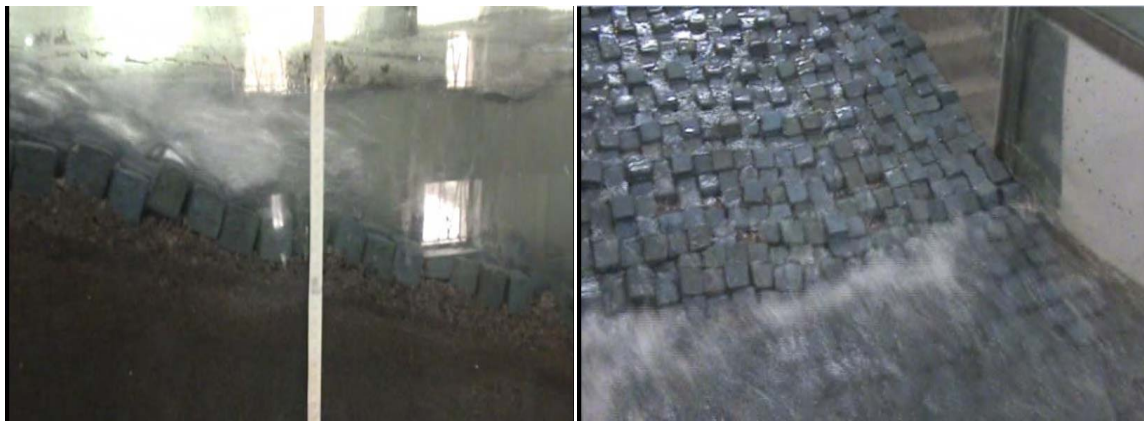
Fig. 4.53 Revetment was stable after Run No 5 (case-2, T=1.5 sec)
