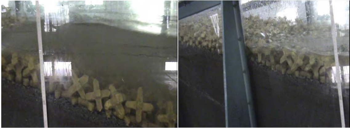
Fig. 4.61 Revetment was stable after Run No 13 (case-4, T=1.5 sec)
