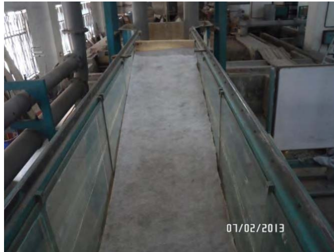
Fig 3.5: Geotextile used as a filter layer
