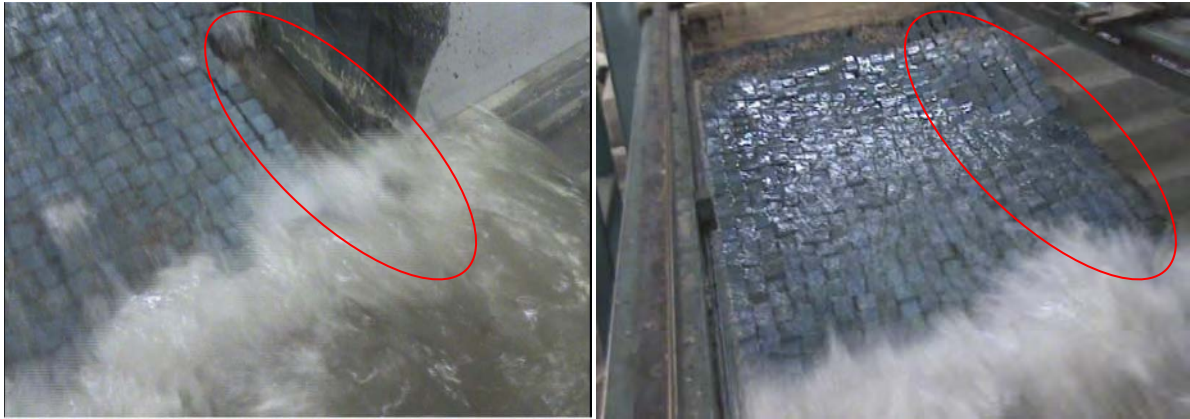
Fig.4. 51 Failure seen at the revetment after Run No 3 (case-1, T=1.8 sec)
