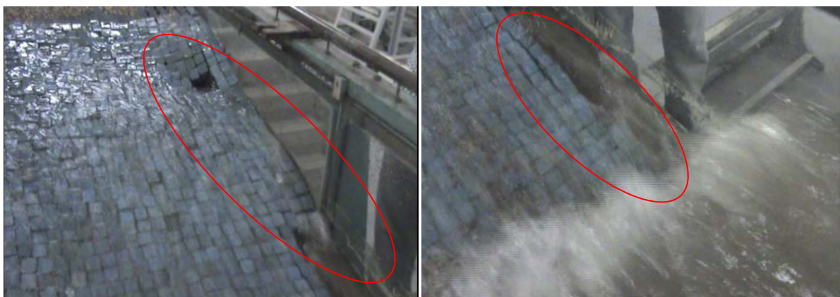
Fig.4. 52 Failure seen at the revetment after Run No 4 (case-1, T=2.0 sec)
