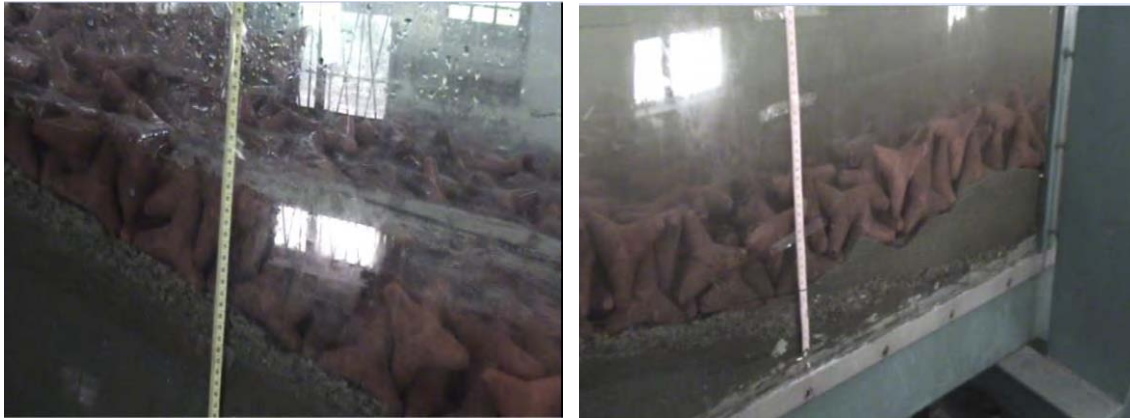
Fig. 4.59 Revetment was stable after Run No 10 (case-3, T=1.8 sec)
