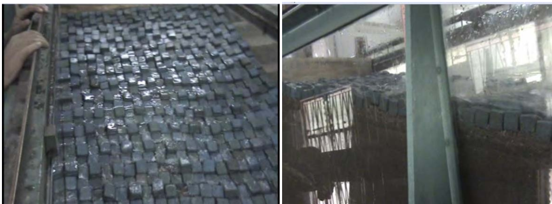
Fig. 4.54 Revetment was stable after Run No 6 (case-2, T=1.6 sec)
