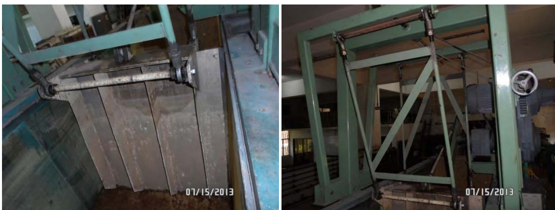
Fig 3.2: Wave paddle with generator
