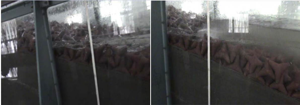
Fig.4.71 Revetment was stable after Run No 23 (case-6, T=1.8 sec)
