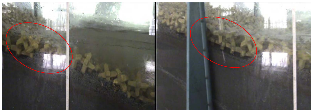
Fig.4.64 Revetment was unstable after Run No 16 (case-4, T=2.0 sec)
