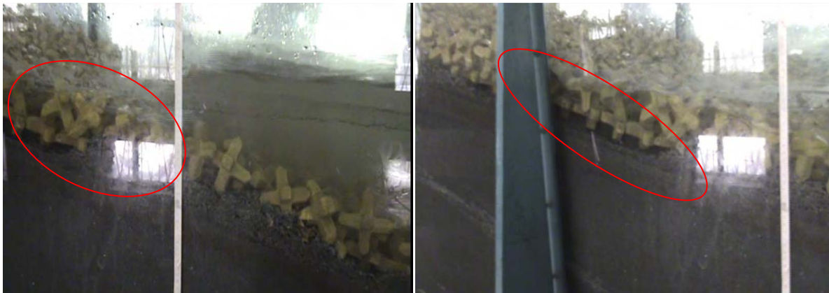
Fig.4.63 Revetment was unstable after Run No 15 (case-4, T=1.8 sec)
