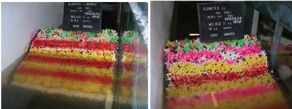
Fig 2.20: After 1000 waves for random placement. After 1000 waves for bundle placement.
