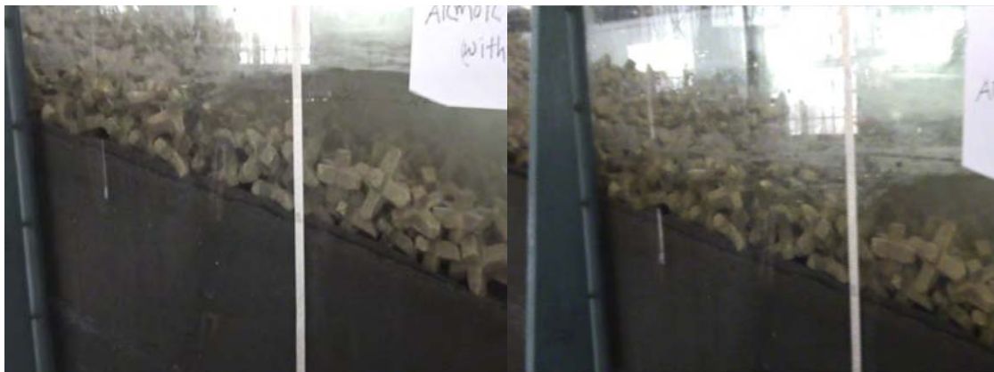
Fig.4.65 Revetment was stable after Run No 17 (case-5, T=1.5 sec)
