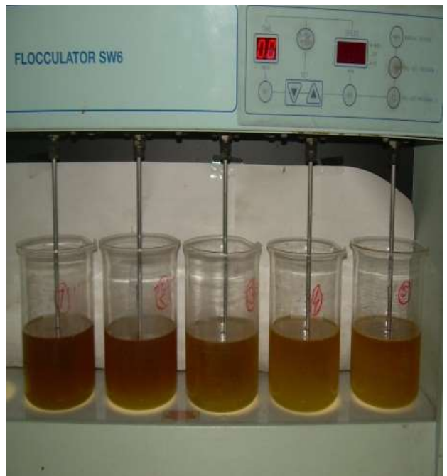
Figure C-8: Samples set in the flocculation unit to accelerate the coagulation process.
