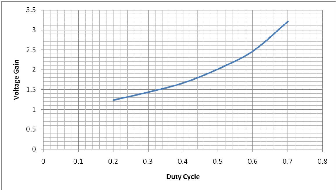
Fig.2.24: Voltage gain vs. duty cycle curve of two switch boost ac-ac converter
