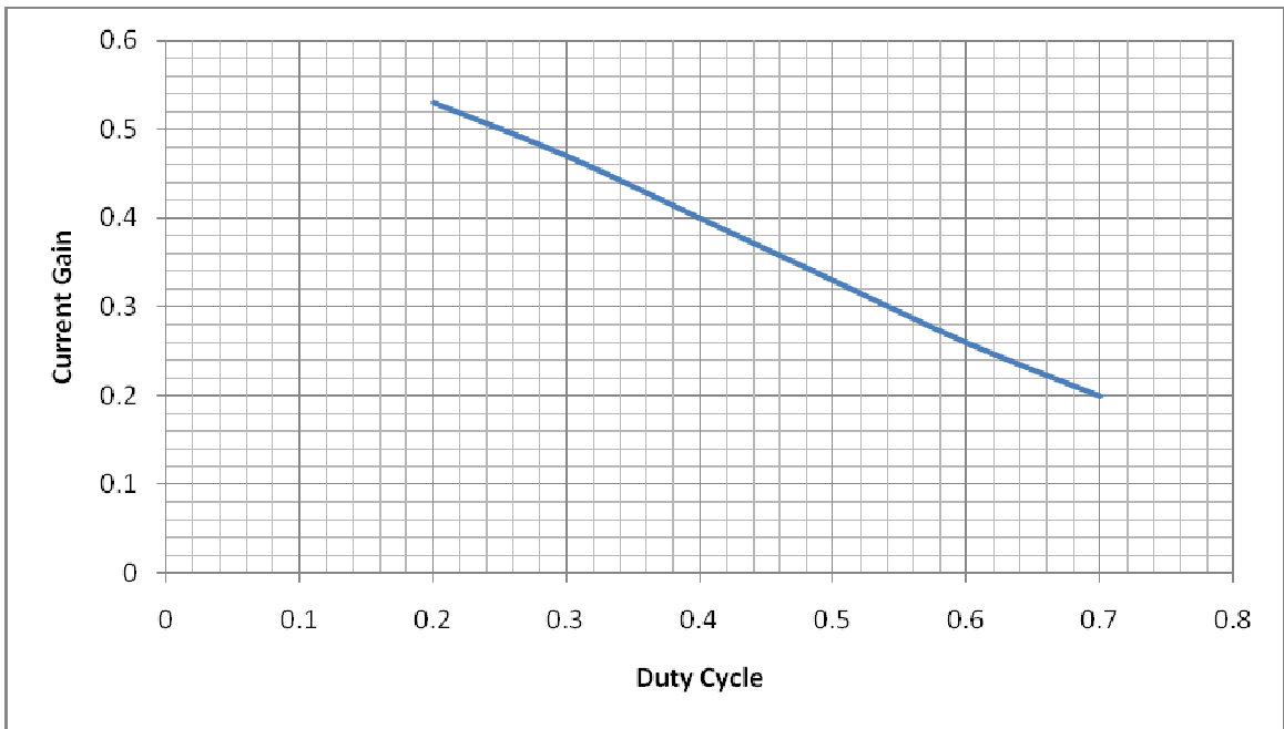
Fig.2.25: Current gain vs. duty cycle curve of two switch boost AC-AC converter
