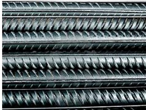
Figure 4.25: Hot rolled steel bars with ribs and oxidized surfaces.
