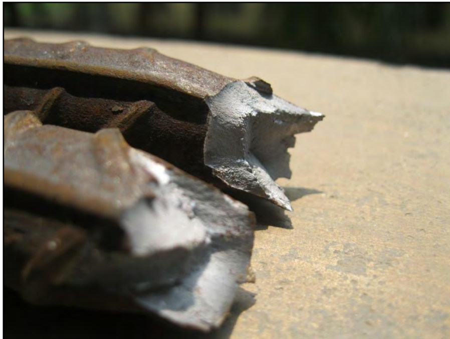
Figure 4.34: Fracture surface of steel 1 with ribs on surface.
