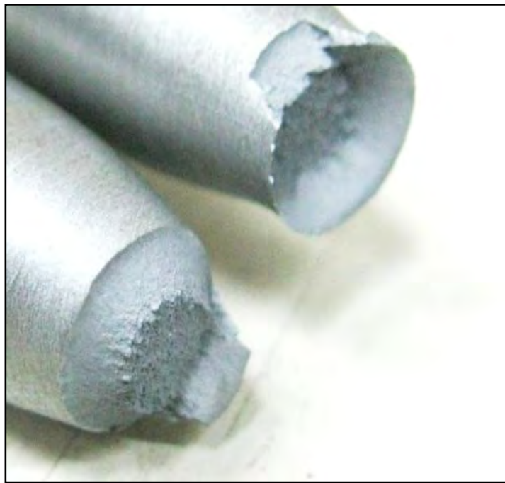
Figure 4.42: Fracture surface of steel 1 without Case.
