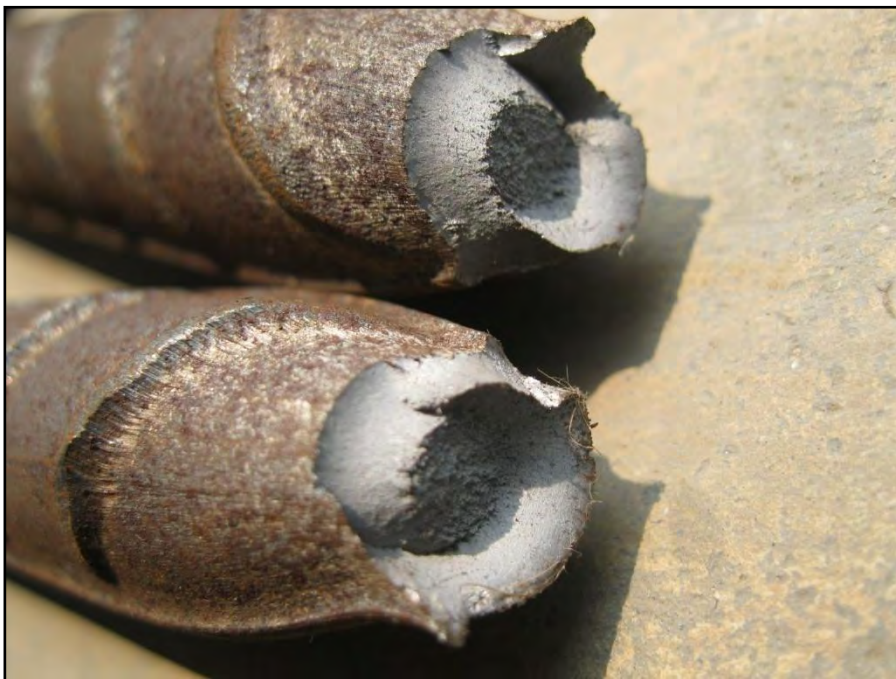
Figure 4.36: Fracture surface of steel 3 with ribs on surface.
