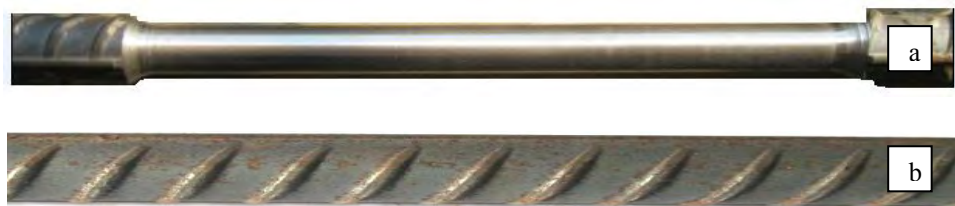
Figure 3.2: The samples of steel rebars prepared for the tensile test (a) removing ribs from the surface and (b) the keeping ribs on surface.
