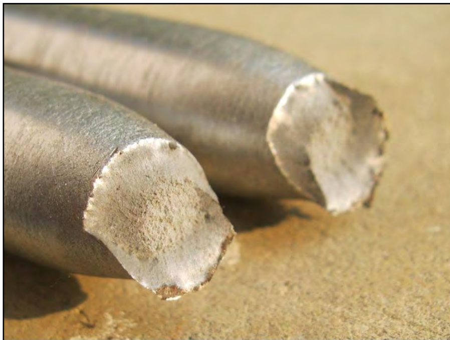
Figure 4.39: Fracture surface of steel 2 without ribs on surface.
