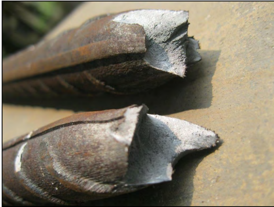
Figure 4.37: Fracture surface of steel 4 with ribs on surface.
