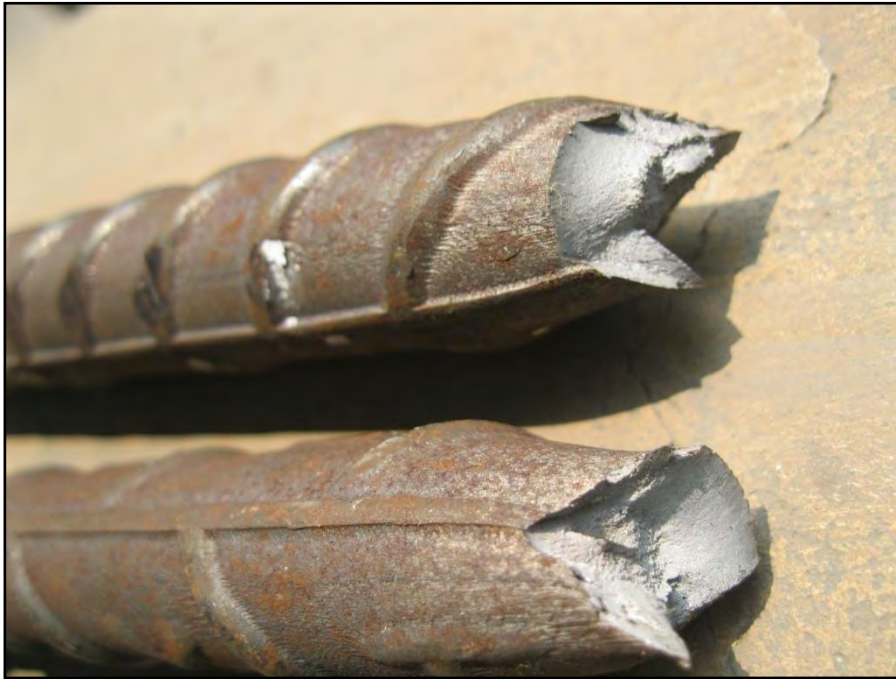
Figure 4.35: Fracture surface of steel 2 with ribs on surface.
