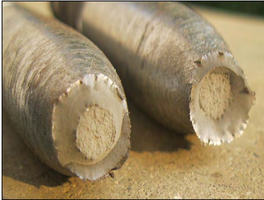
Figure 4.40: Fracture surface of steel 3 without ribs on surface.
