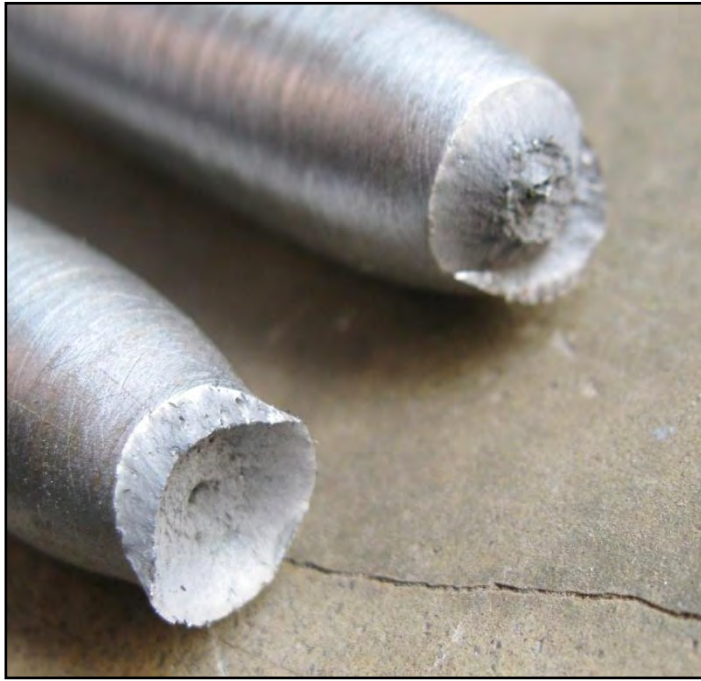
Figure 4.45: Fracture surface of steel 4 without Case.
