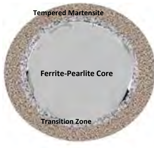
Fig.2.1: The structure of the QT/TMT steel with Tempered Martensite Case, Ferrite-Pearlite Core and Transition Zone middle of the Case and Core [11].
