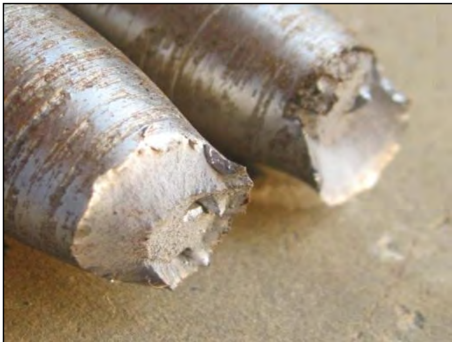
Figure 4.41: Fracture surface of steel 4 without ribs on surface.
