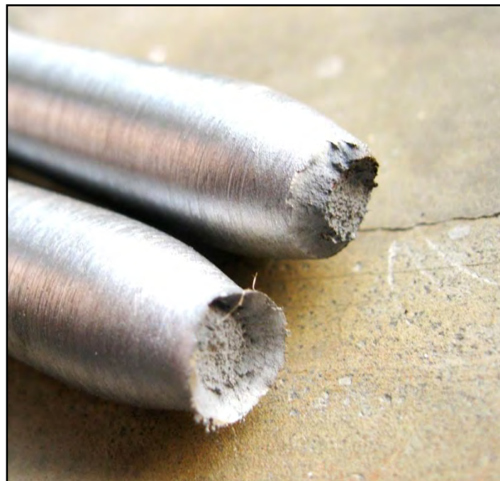
Figure 4.44: Fracture surface of steel 3 without Case.
