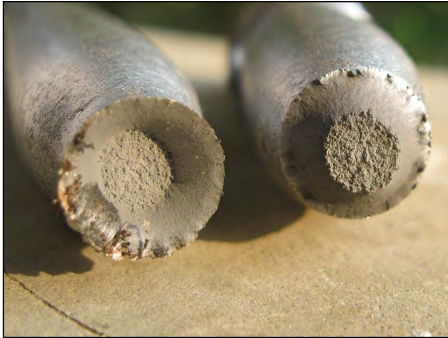
Figure 4.38: Fracture surface of steel 1 without ribs on surface.
