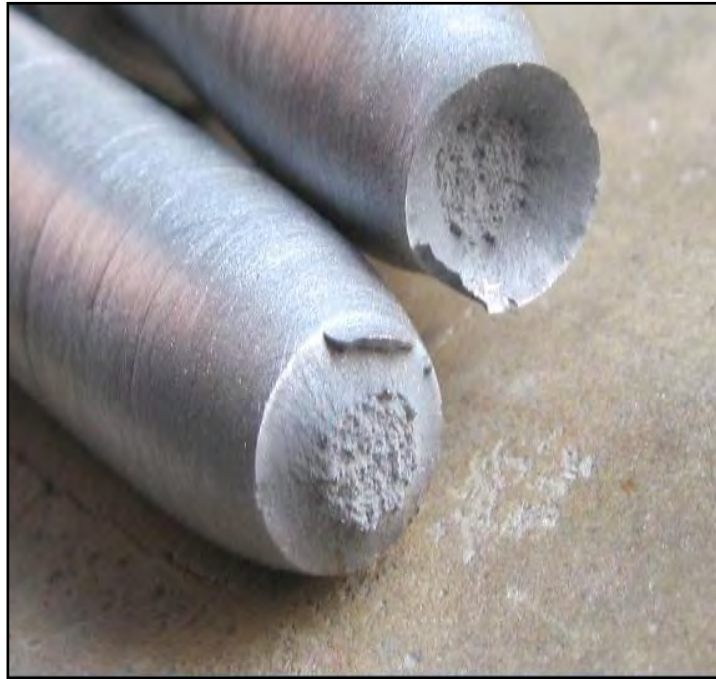
Figure 4.43: Fracture surface of steel 2 without Case.
