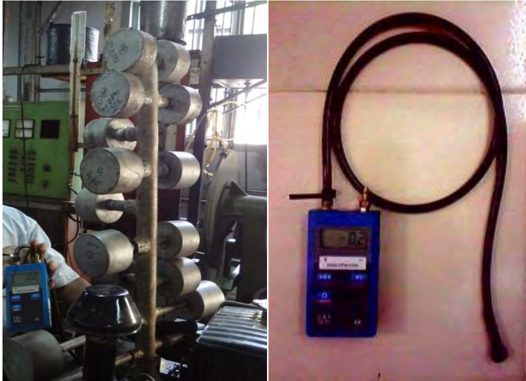
Fig B-3: Measurement of exhaust back pressure by Differential pressure gauge
