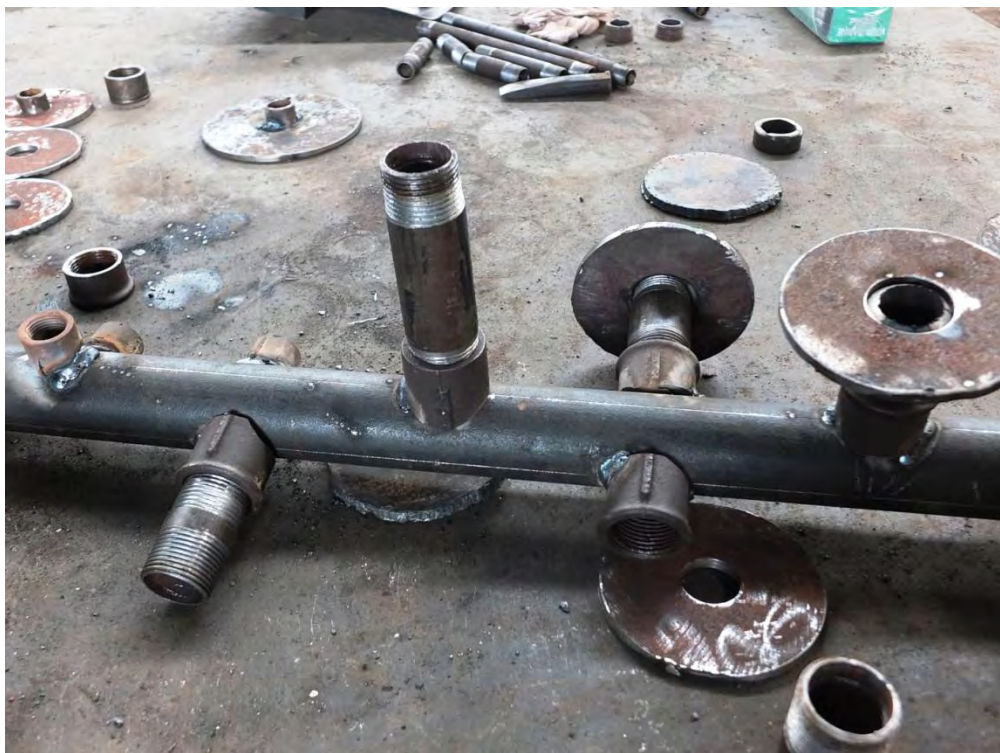
Fig B-1 Modified Helmholtz resonator fabrication in the workshop
