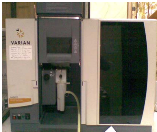
Fig. 3.8 Atomic Absorption Spectroscopy (VARIAN AA240 FS)
