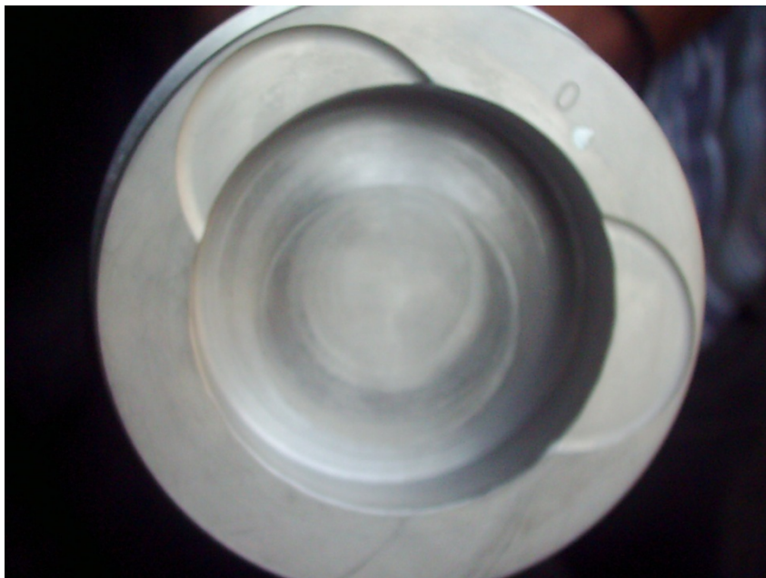
Figure 3.54: Post machining piston top view (CR=12)
