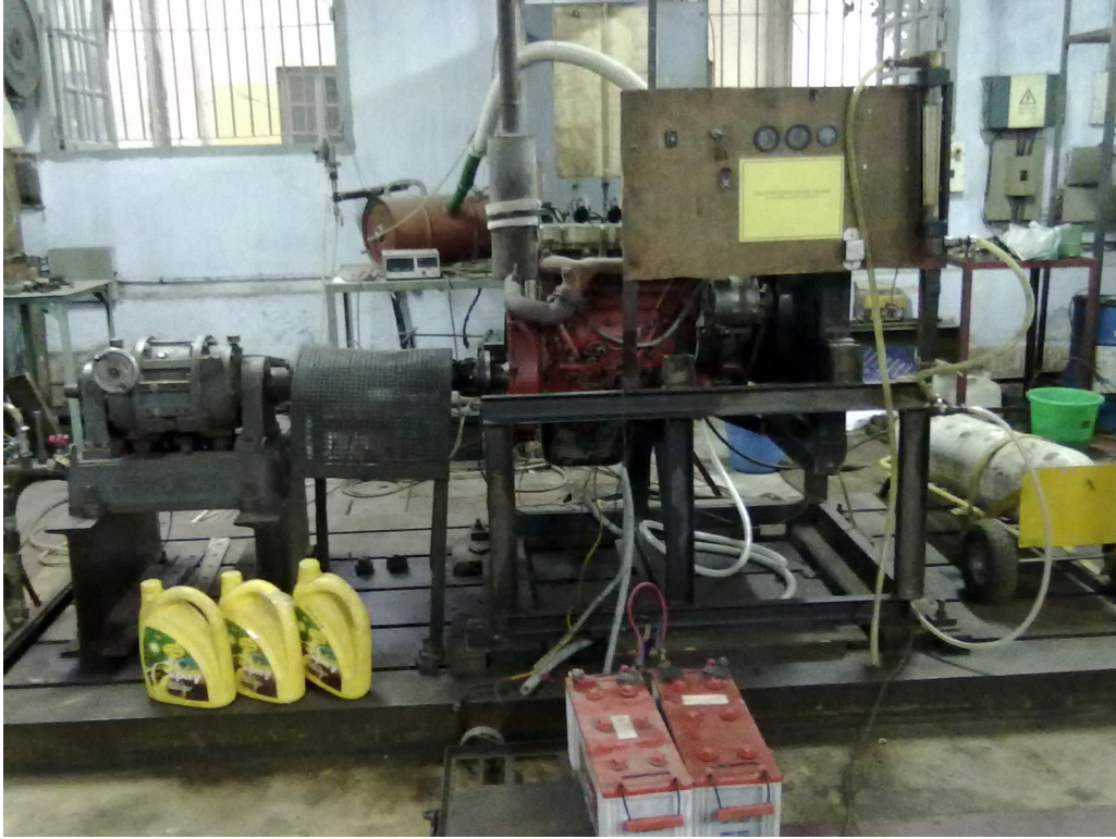
Figure 3.32: Experimental Setup (CNG converted diesel engine)
