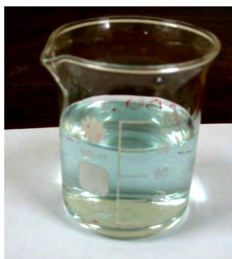
Fig 4.29: Residual solution after sulphuric acid washing of Kuakata sand
