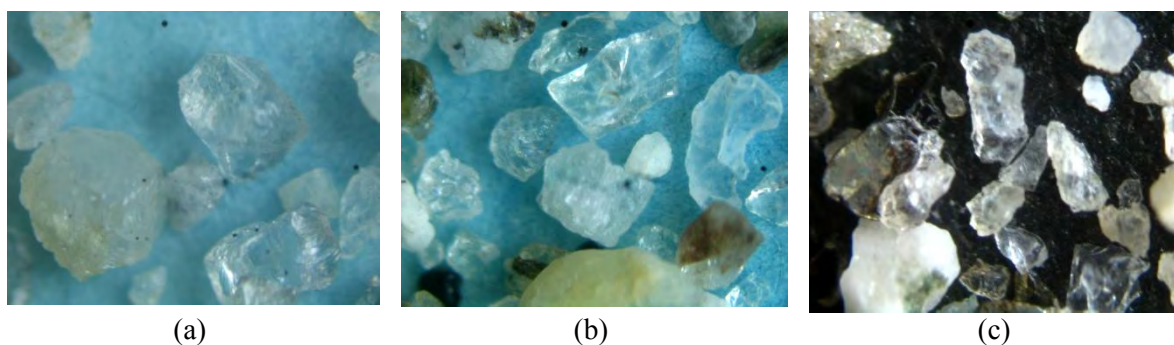
Fig 4.25: Acid washed sample of Patgram with 192x magnification (a) 10% HCl, (b) 15% HCl, (c) 20 % HCl. (Percentage of original width x height: 18 %.) Increment in acid concentration beneficiates the sample.
