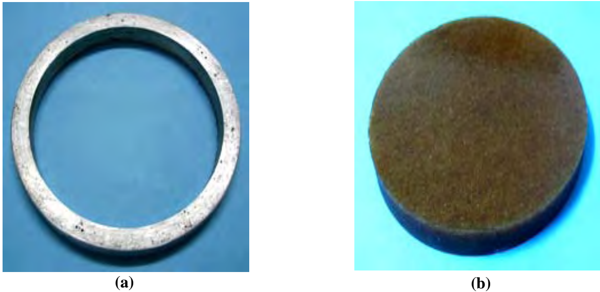
Figure 3.7: Photographs showing the (a) casting mould, (b) as cast sample
