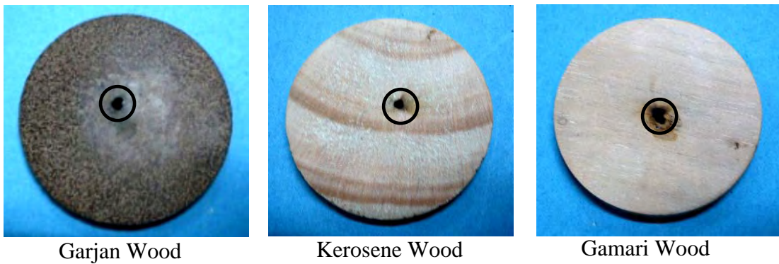
Figure 4.16: Various wood samples after breakdown voltage test. Note: During breakdown voltage test burning caused large size pores in all wood samples (marked by circles).
