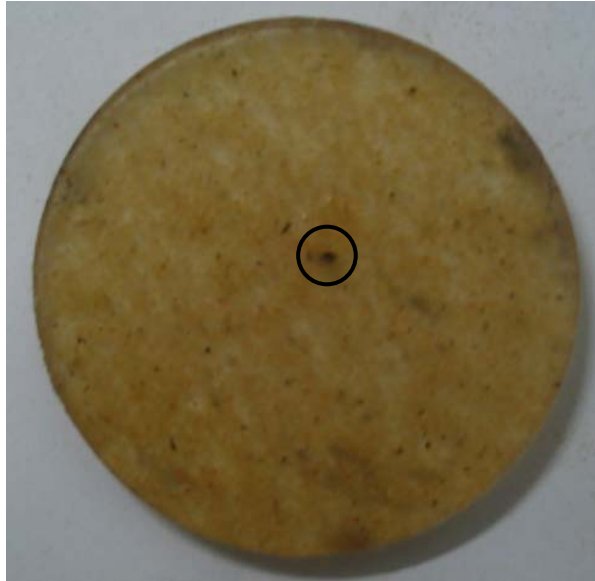
Figure 4.18: Photograph showing a typical pore created during breakdown voltage test of a composite sample.
