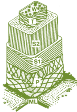
Figure 2.7: Transmission electron micrograph of a vascular cell (softwood tracheids, hardwood libriform fibers). Middle lamella (ML), primary wall (P), S1, secondary wall 1 (S1), secondary wall 2 (S2), tertiary wall (T) and warty layer (W) [73].
