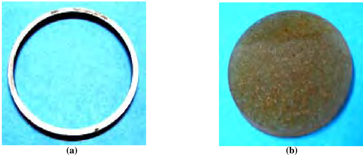
Figure 3.5: (a) Picture of casting mould and (b) test sample for breakdown
