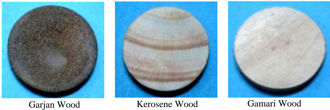
Figure 4.15: Samples of various woods before breakdown voltage test.
