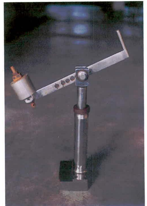
Figure 3.4 : Construction of load arm.
