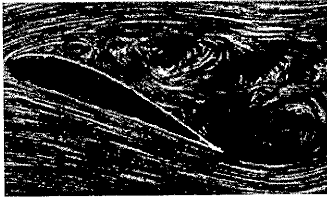
Figure 2.2: Flow separation on an aerofoil shape which is at high angle of attack (Source: http://www.nationmaster.com/encyclopedia/Flow-separation )
