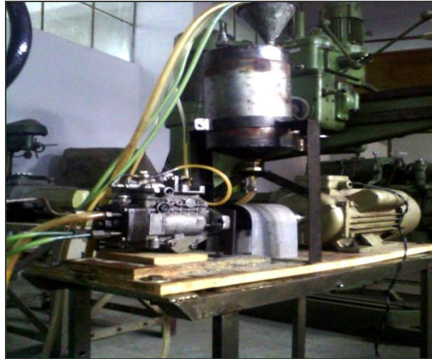
Fig.2.1 Photographic view of MQL setup
