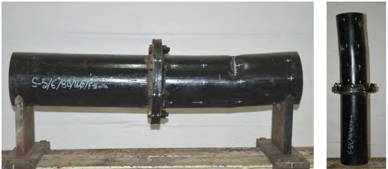
Figure B18: Deflection of 150 mm pipe with 8- 16 mm bolts and 14 mm flange(S-5)
