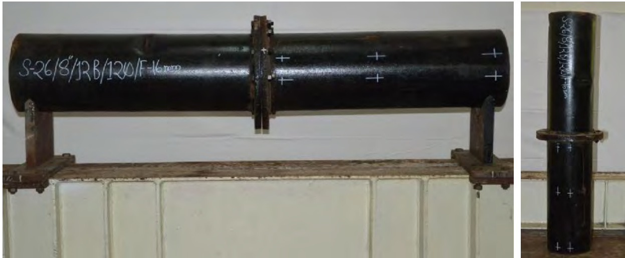
Figure 4.6 (a) Deflected shape of a 200 mm diameter pipe with 16 mm flange thickness (S-26) showing effect of flange thickness on deflection
