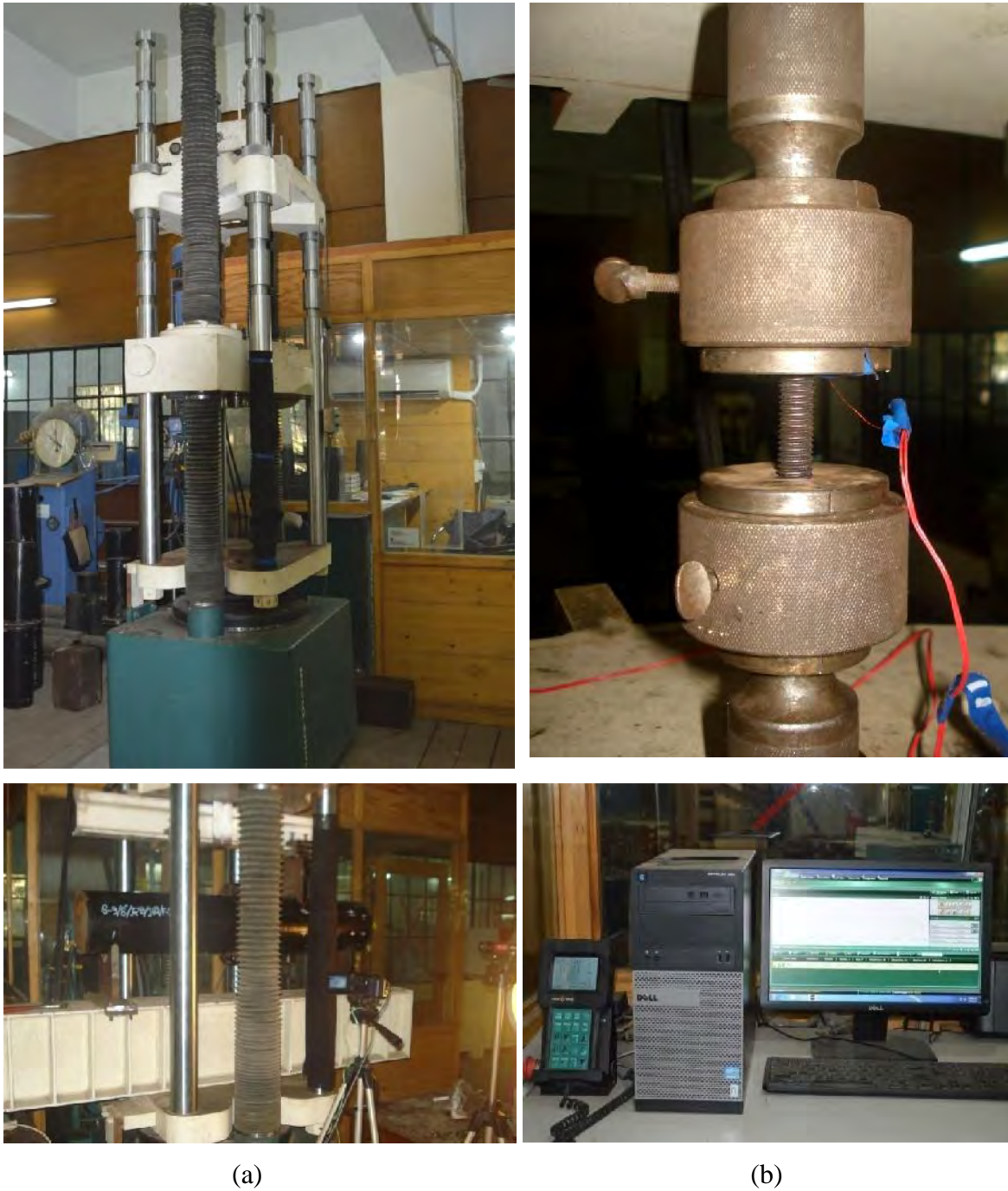
Figure 4.3 (a) Tinious Olsen universal testing machine (UTM), (b) Direct tension test of bolt and Control panel for monitoring UTM operation
