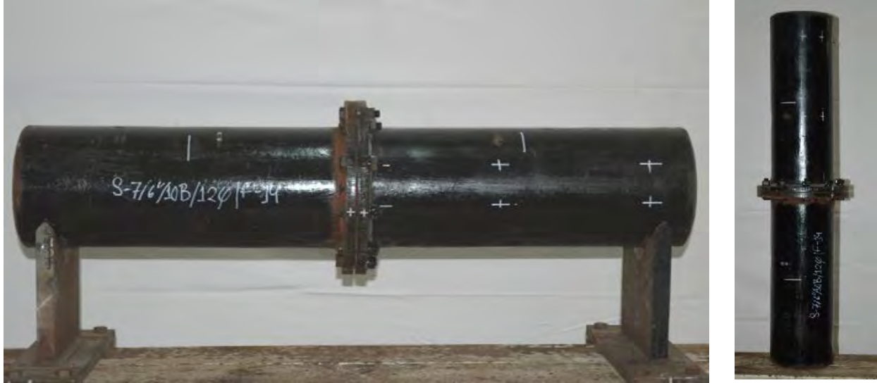
Figure B17: Deflection of 150 mm pipe with 10- 12 mm bolts and 14 mm flange(S-7)
