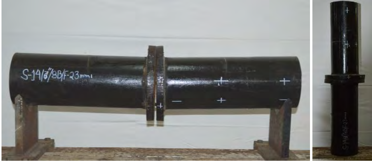
Figure B19: Deflection of 150 mm pipe with 8- 12 mm bolts and 21 mm flange(S-14)
