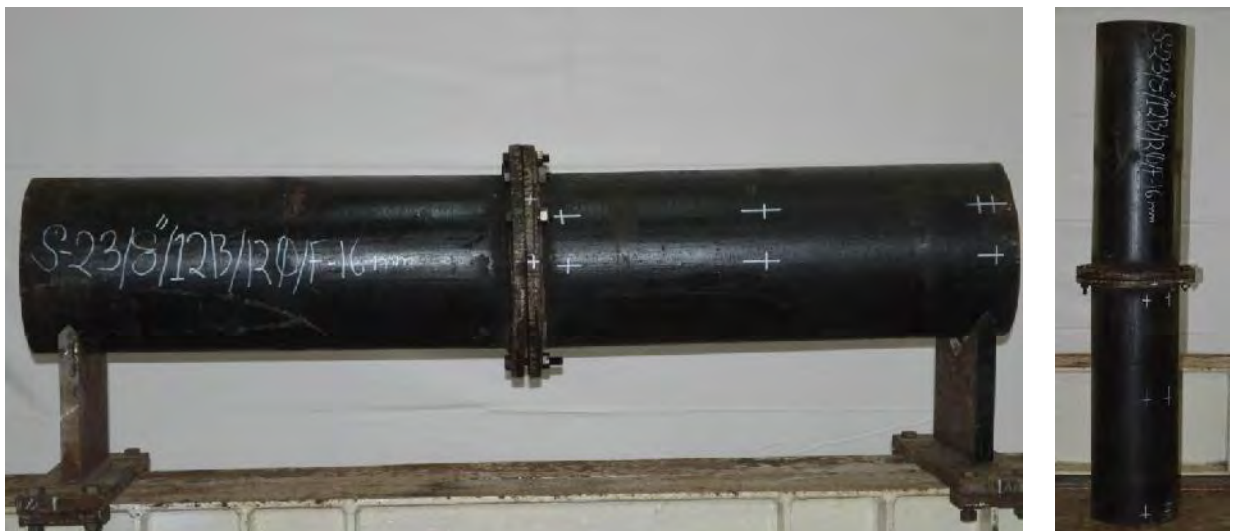
Figure B28: Deflection of 200 mm pipe with 12- 12 mm bolts and 16 mm flange(S-23)
