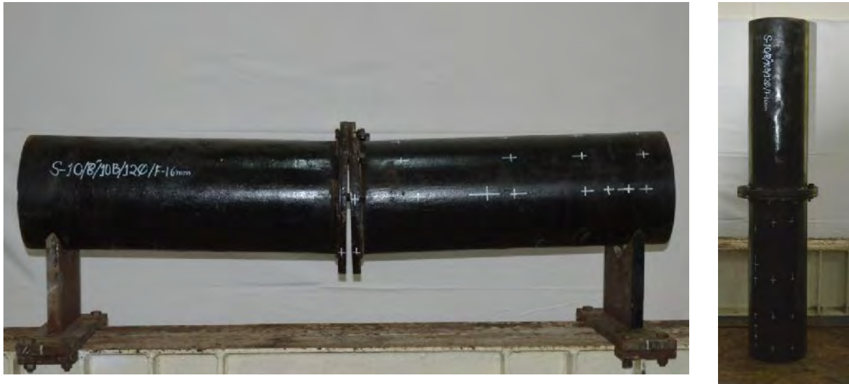
Figure B27: Deflection of 200 mm pipe with 10- 12 mm bolts and 16 mm flange(S-10)
