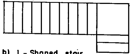
(b) L-Shaped stair with landing
