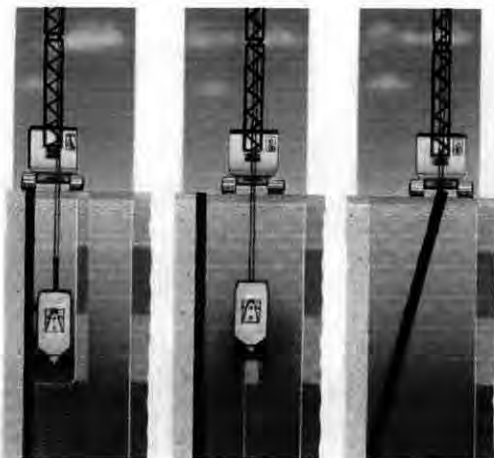
(1) Diaphragm wall excavation
