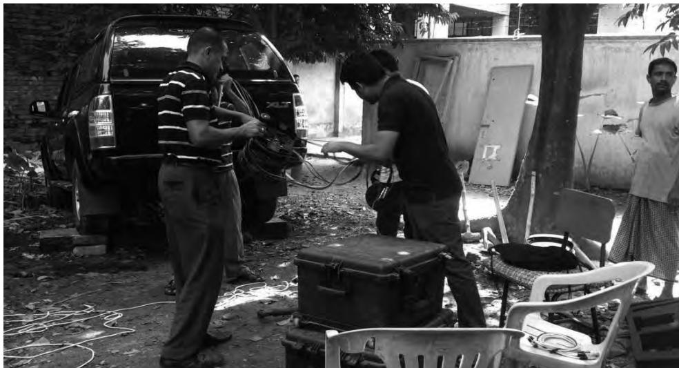
Figure 3.7 PS Logging Test Setup at Gulshan-2, Dhaka.
