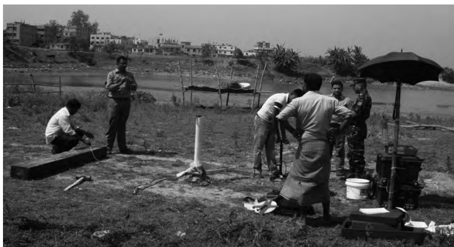
Figure 2.14 Seismic down-hole test at MIST
