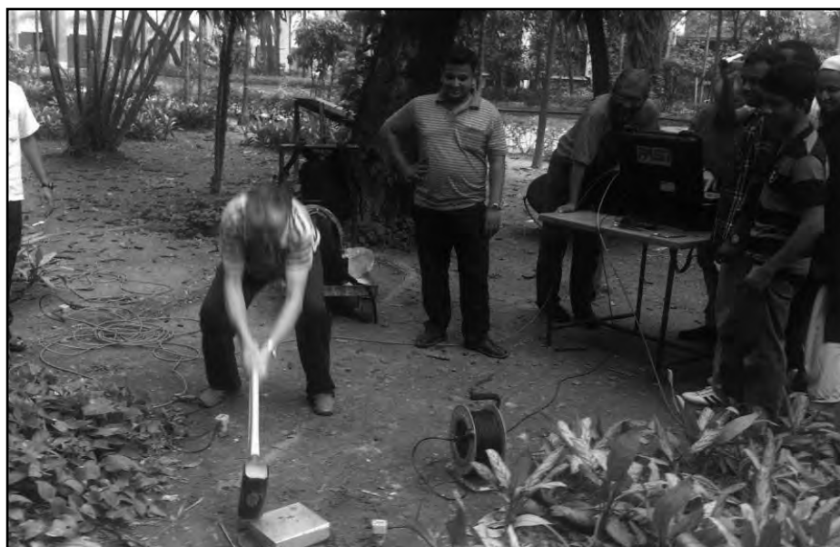
Figure 2.7 Seismic Refraction survey in BUET.
