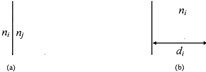
Figure 6.19 Two basic elements used in forming the transfer matrices: (a) Interface between two media with different refractive indices n_i and n_j and (b) layer with refractive index n_i and thickness d_i .
